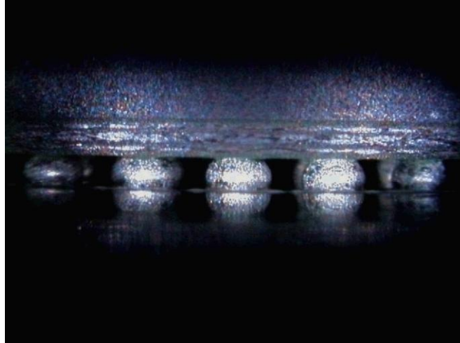
Figure 8.5. Edge View Camera Inspection
