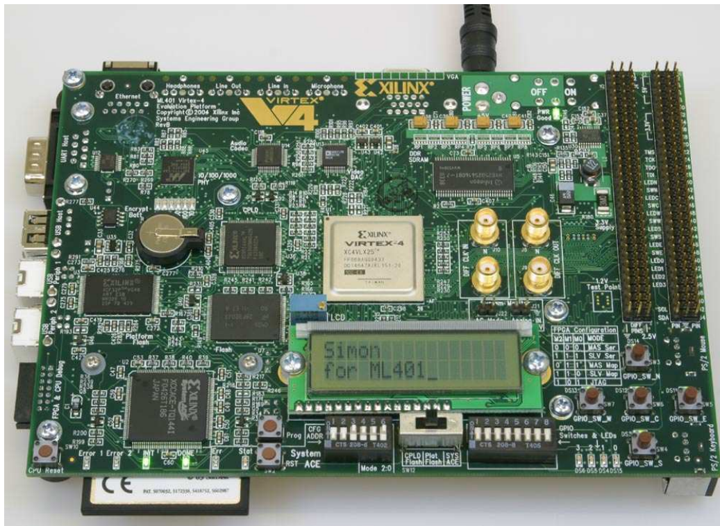
Figure 7.3. Xilinx ML401 development board.
