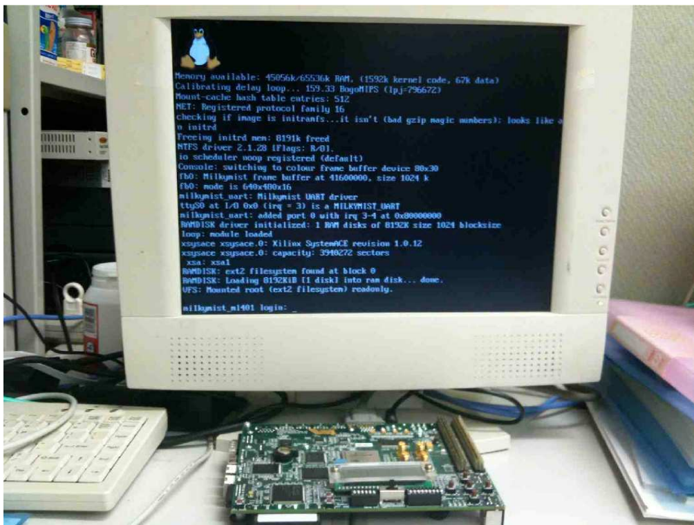
Figure 7.2. Linux booting on the Milkymist SoC.
