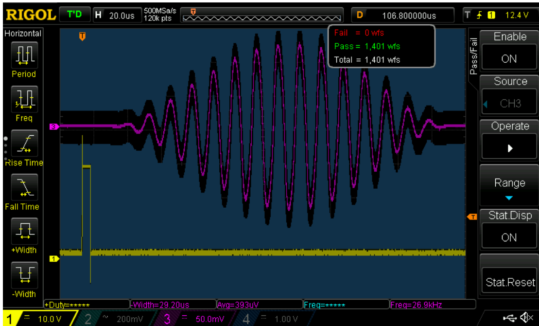
Figure 3.16: STFT pulse generator timing test. The oscilloscope is triggered on the yellow TTL pulse and checks if the purple STFT pulse falls within the configured mask. The pulse is configured to be a single frequency, shaped by a Hann window. No timing errors are reported after 1400 tries.
