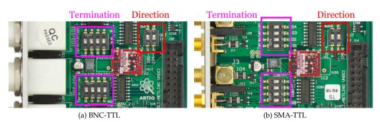
**Figure 5: Position of switches**
