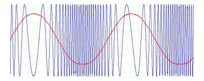
The frequency variation is greatly exaggerated. Red represents the encoded sound wave.
